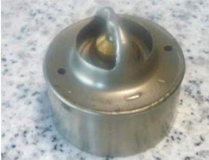
An automotive thermostat modified for use with a Model A. Note the skirt welded to the base to prevent it from tumbling in the water outlet hose. Two small holes are drilled into the base for a small amount of water flow when the thermostat is closed.
