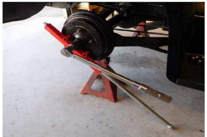
A torque wrench is shown positioned on the rear axle nut to tighten it.
