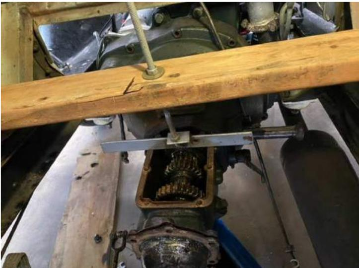
One shot you can see my rear heavy duty rubber engine mounts also, actually off a big helicopter, I added two lateral composite blocks to stop the engine moving laterally to reduce steering wander. If anyone's interested I can show closer detail and have two of the mounts spare.
