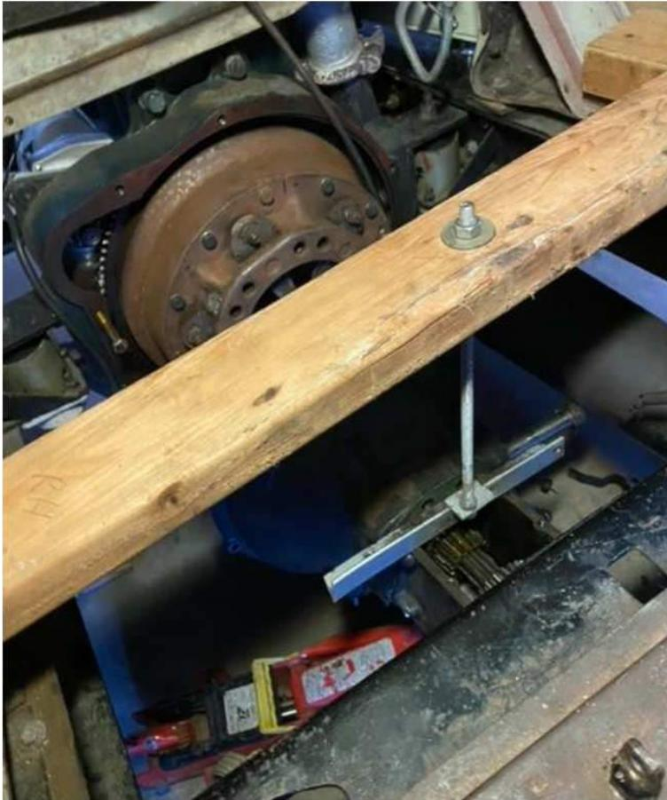
I fabricated two bits of 4 x 2 and laid one down either side of the chassis, chiseled out slots for the body mounting bolts. Then a length from side to side and drilled a hole in the center for the 10mm threaded rod. Drilled a piece of angle to bolt to the front top cover holes and a hole through the center for the threaded rod. Double nuts on the angle end of the rod. A third nut for lowering the gearbox.
