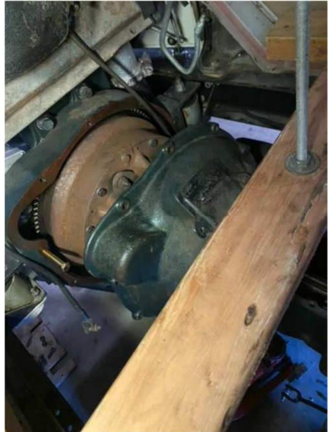
Unbolt the bell-housing, slide the cross piece of 4x2 back and lower slowly to the floor. Refitting the same way using a couple of bell housing spigots made out of two long bolts with the heads chopped off. Slow but easy.
