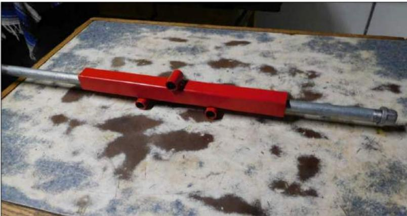
The tool is shown here. It is mounted on the brake drum so that three lug bolts on the brake drum are inserted into the three tubes on the tool. The pipe is then extended down through the tool to rest on the ground to prevent the drum from turning as the axle nut is being torqued.
