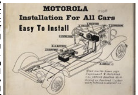
A Motorola car radio installation diagram (circa 1930) showed batteries, spark plug suppressors and the antenna, in addition to the radio components.
