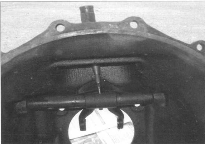
Photo 1 - Remove the radius ball components and orient the pin to the opening to drive out the pin.
