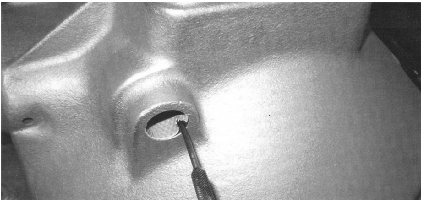
Photo 3 - Remove the old bushing by driving a sharpened punch under the bushing. The entire housing was sandblasted to prepare for painting.
