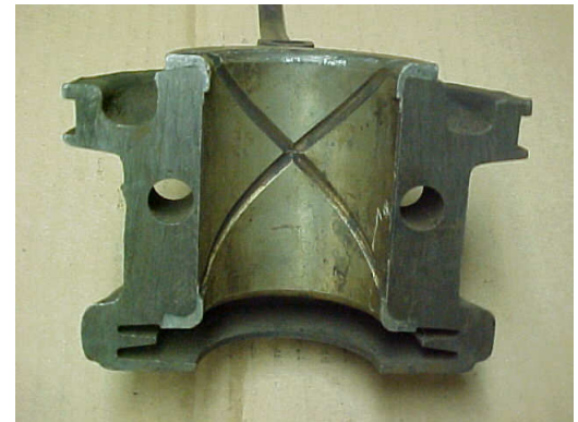
NOS Cap Showing Original Babbitt Thicknesses
