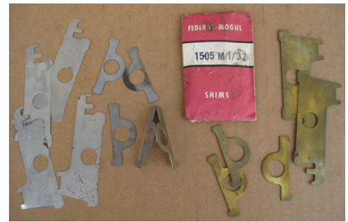
Original thin steel shims on the left, vs. thick laminated brass shim packs on the right
