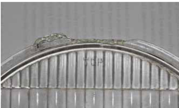
Even a fairly large fracture can be repaired with this Method. Here it is filled a little extra at the upper edge to prevent water intrusion, and the lip has been moved slightly to the left compared to the original location. And it does not matter, doesn't seem to anyway.
