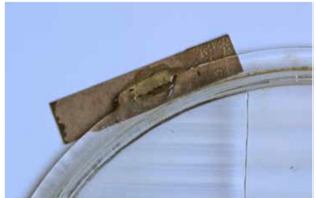
At the first attempt and by training in the technique, it can be helpful in putting a piece of cardboard during the build-up point. Remove afterwards and scrape away scraps of cardboard
