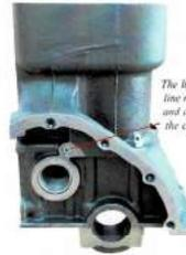
The hidden oil line runs fore and aft inside the chamber.
