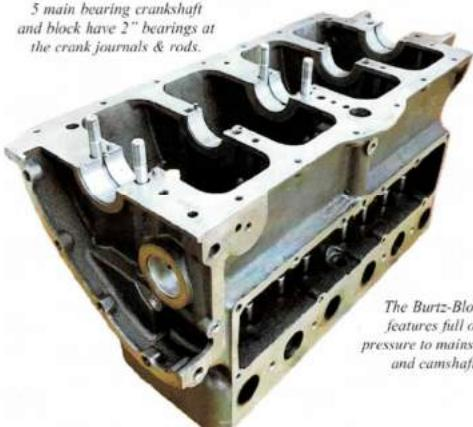
The Burtz-Block features full oil pressure to mains, rods and camshaft.
