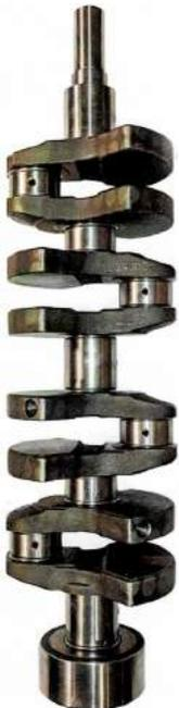
5 main bearing crankshaft and block have 2" bearings at the crank journals & rods.
