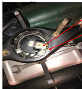
Distributor Rotor Distributor body, cylinder number #1 contact pin
