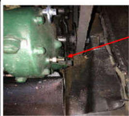
Timing pin taken out And re-inserted with Threads facing out
