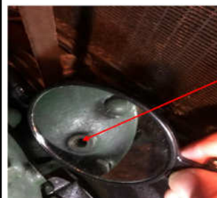
Dimple on timing gear shown in timing pin hole, dimple will appear black on the timing gear
