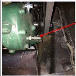
Timing pin (threaded into the Timing cover)
